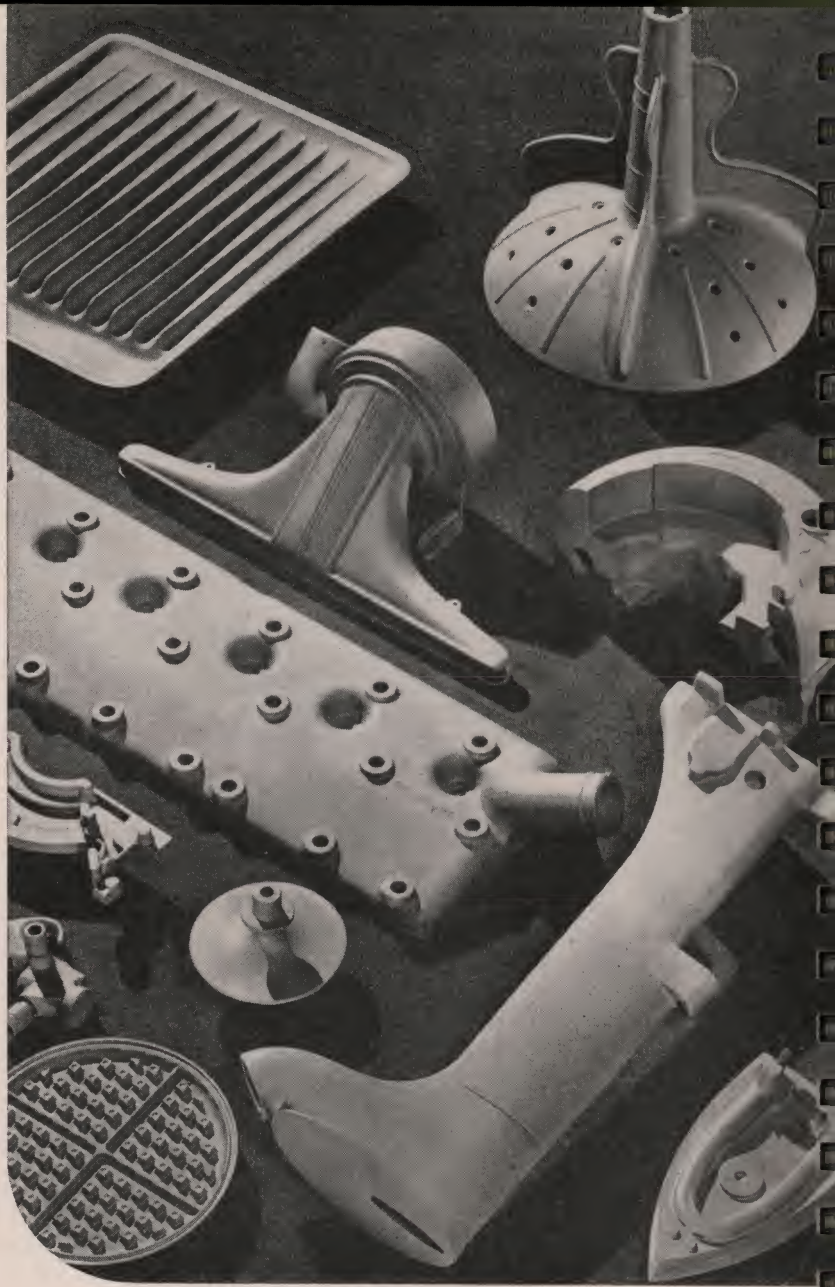
Aluminum permanent-mold and semi-permanent-mold castings.
